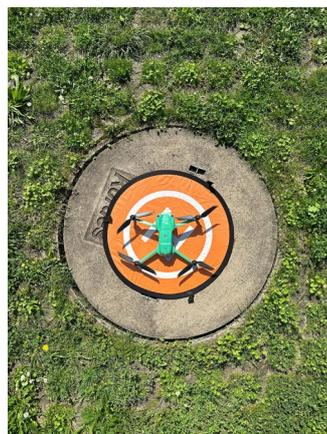
Avoid taking off from a surface with metal (e.g. reinforced concrete), as this interferes with the drone's compass.
