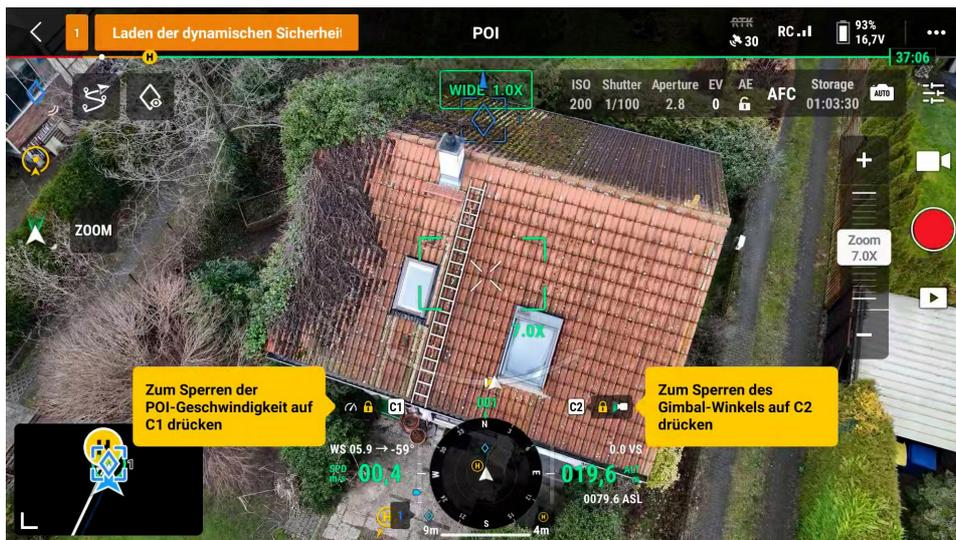
To freeze the speed, you must first accelerate the drone. In POI mode, you can only move the drone in a circular path; all other directions are blocked. So you move the right stick of the controller very slightly to the left or right (depending on the direction in which the circular flight is to be performed). The further you move the right stick in one direction, the faster the drone accelerates. At the moment when the speed reaches 0.5 m/s, you can freeze it by pressing the C1 button.
