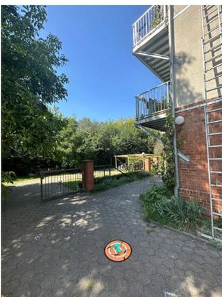
Too close to the building - If the drone is too close to the building, the quality of the satellite connections decreases, and the drone takes a very long time to find 12 or more satellites.
