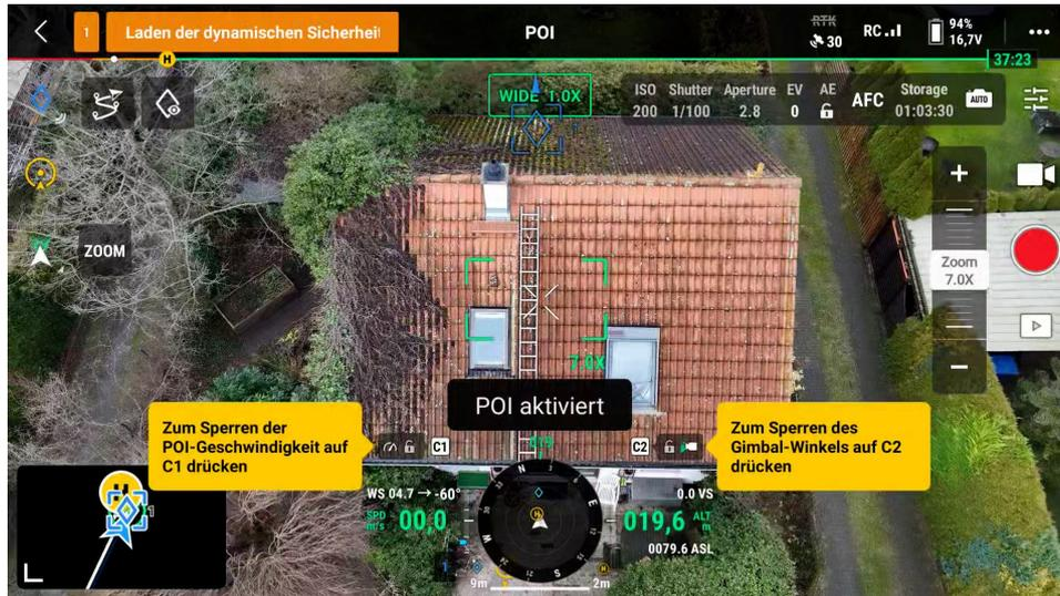
As you can see from the illustration, you now have two new settings. You can now use the drone's "C buttons" to freeze the speed and the camera angle.
