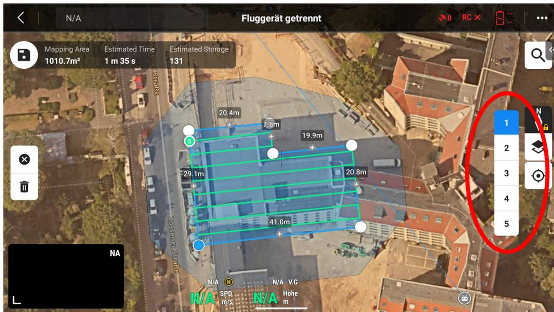
The first flight path runs directly over the building when set up correctly. The other 4 flight paths are then next to and partly above the building, as can be seen in the following screenshots!
