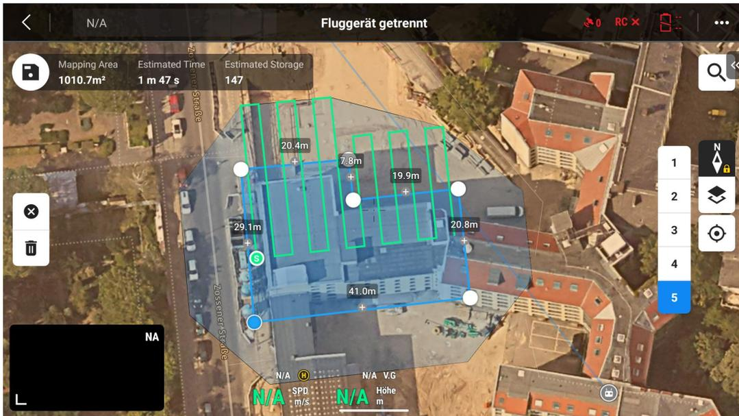
If all 5 paths are now viewed together, the drone first flies over the entire roof and then flies over the building once from each direction. In this way, all edges and the roof are captured from different perspectives. This is ideal for obtaining an optimal 3D model and the best quality data.
